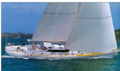
SORCERER II 28.95m/94'9", Cookson, 1998 Quick acceleration, responsive and fast, Frers design and light weight composite hull, carbon (Southern Spars) rig and furling boom.
