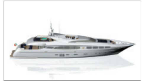
MONDOMARINE 41m/134'5, Mondomarine, 2008 41m aluminium semi-displacement hull designed by Cor D Rover. She can achieve 20 knots maximum speed and 17 knots cruising. Transatlantic range.
