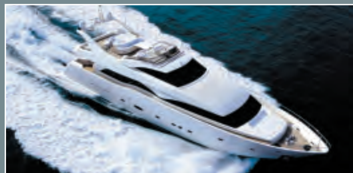
VANILLA 28.8m (94.49) Ferretti, 2002 The 28.8m Vanilla is one of the few vessels of her size with the owner's cabin on the main deck. She is a substantial fast flybridge yacht with good sea-keeping qualities. She is well equipped and powered by twin MTU 2000 engines.
