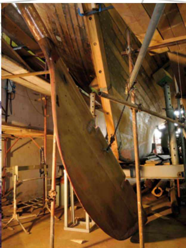
This page & opposite: Eilean's frames had to be replaced one by one before she was transported to the restoration yard in Viareggio, where work on new riveting, beams and deck structure were completed. Work has begun on her masting
