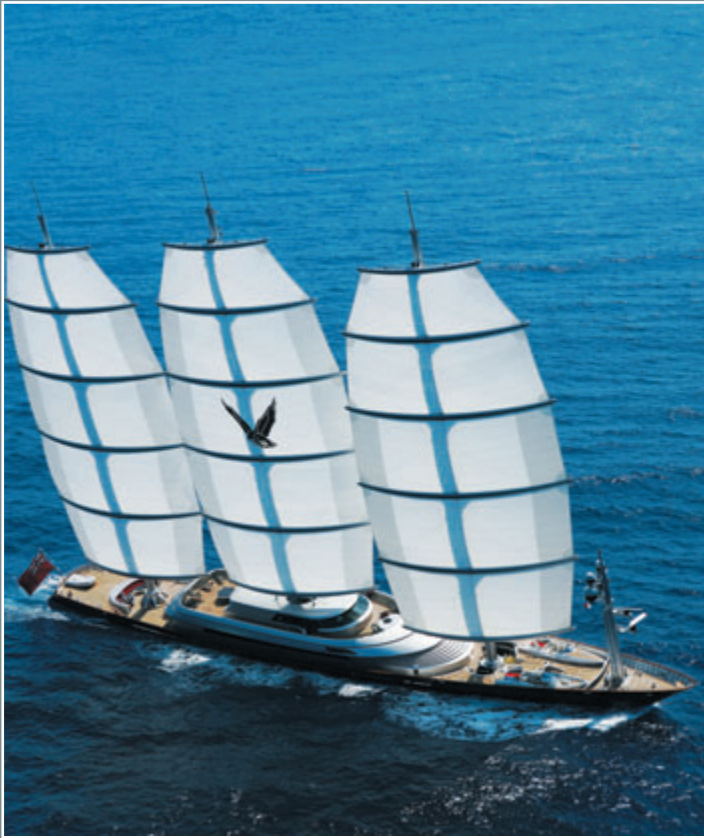
MALTESE FALCON 88m/288.8', Perini Navi, 2006 Maltese Falcon represents a true breakthrough in yachting with her unstayed carbon fiber rotating "Falcon Rig" and unique fully retractable sails coming out of, and disappearing into, the carbon masts. She is the crème de la crème of superyachts and the finest contemporary sailing yacht built.
